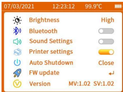
**Screen brightness:** After the instrument is turned on for 5 minutes without operation, the instrument automatically reduces the brightness to save power, press any key to restore the set brightness.
