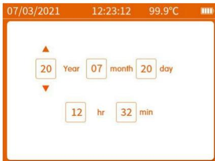
The time setting interface is used to calibrate the instrument time. After entering the time setting interface, press the "◀" or "▶" key to move the cursor, press "▲" or "▼" key to modify the time and date parameters. After setting, press "⏪" key to save the actual setup.
